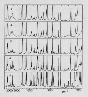
Raman spectra of ethyl benzoate: a liquid, b amorphous solid, c crystal B, d crystal A, e crystal C
